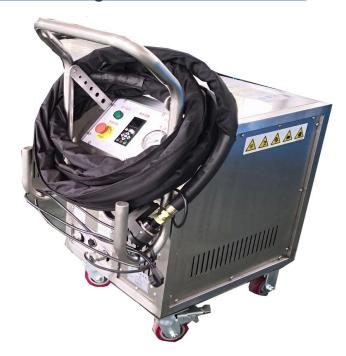
The Magicball YGQX-750 Dry ice blasting machine cleaning with dry ice! This new development is quickly expanding around the world. One system uses small rice size pellets of dry ice shooting them out of a jet nozzle with compressed air. It works some what like sandblasting or high-pressure water or steam blasting, with superior results. The frigid temperature of the dry ice is  $-78\,^{\circ}\text{C}$ .
